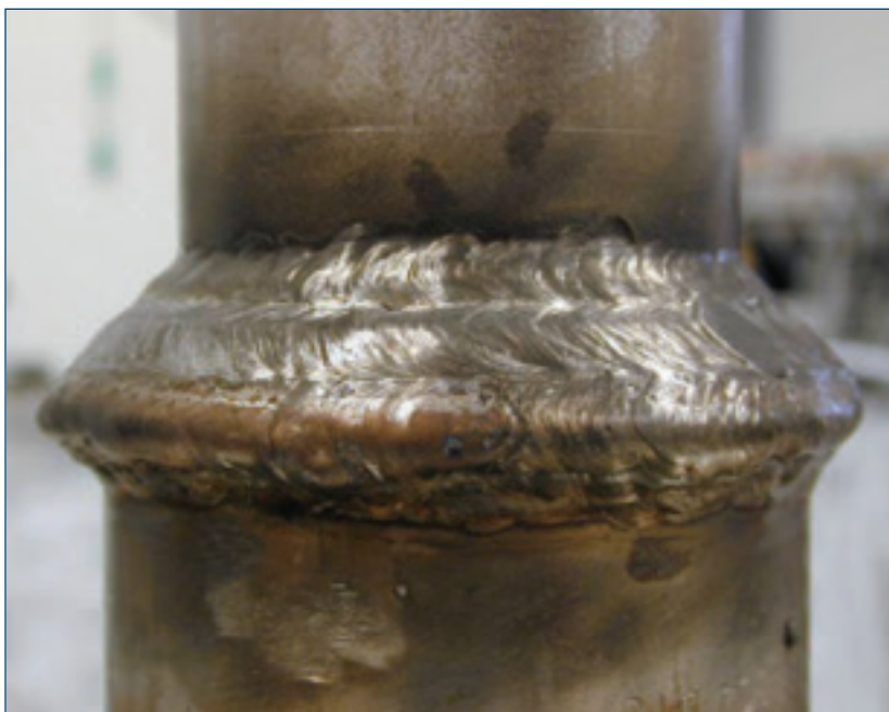
Fig. 4 — Socket weld repaired by weld overlay.
