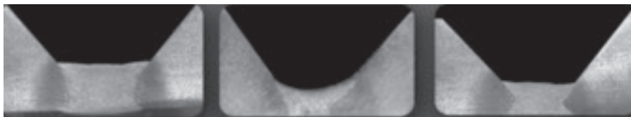
Fig. 1 — Comparison of root passes performed by modified short circuit GMAW (left), GTAW (center), and traditional short circuit GMAW (right).
