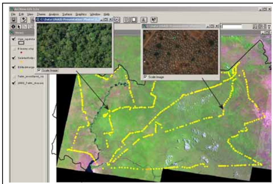
Figure 3.2 Flight routes taken for the northern Uganda Aerial survey showing two example photos from the collection taken every 2 minutes.
