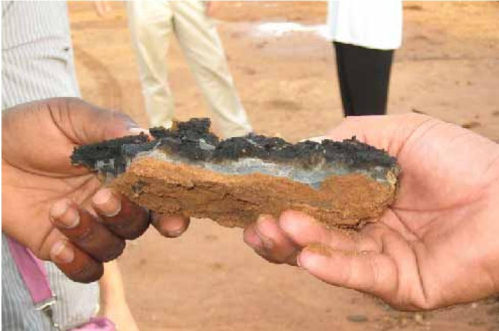
**Photo 3: lighter grey bentonite layer in sample from excavated waste pit at Mputa-1**
