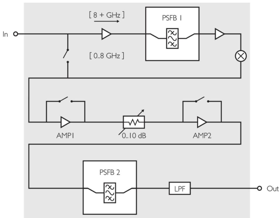
Figure 1: R5500 Real-Time Spectrum Analyzer Front-End Block Diagram
