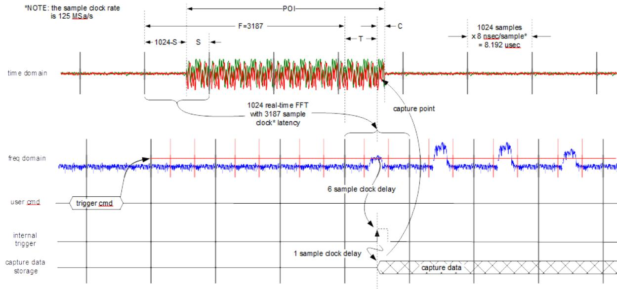
Figure 2: ThinkRF RTSA's Triggering Mechanism Waveforms
