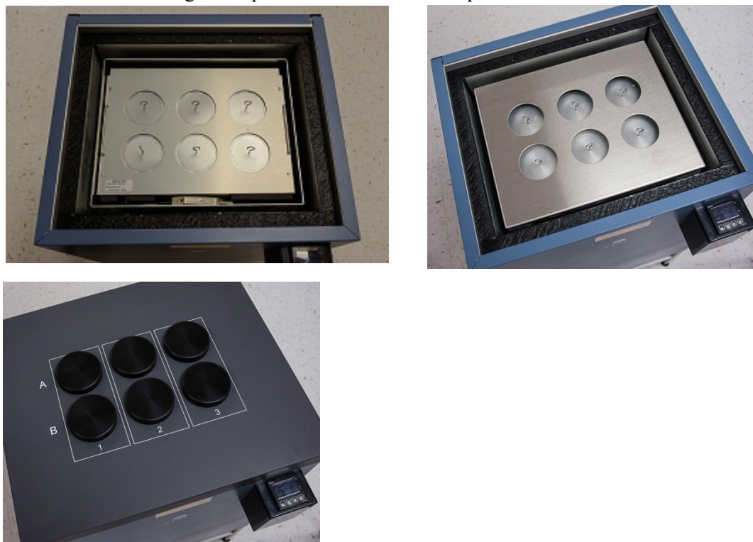
Figure 25 Lower calorimeter block in center of TAM air cavity (top left); Place matching sheet metal panel (top right) and lid (bottom left) onto the TAM Air.
