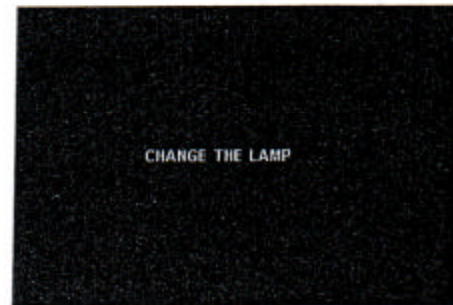
Figure 18 Lamp replacement warning signal II
