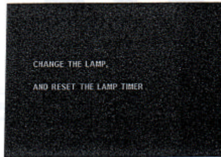
Figure 16 Lamp replacement warning signal
