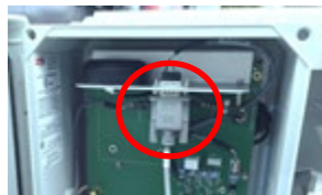
Figure 2-2: Command port serial cable connection
