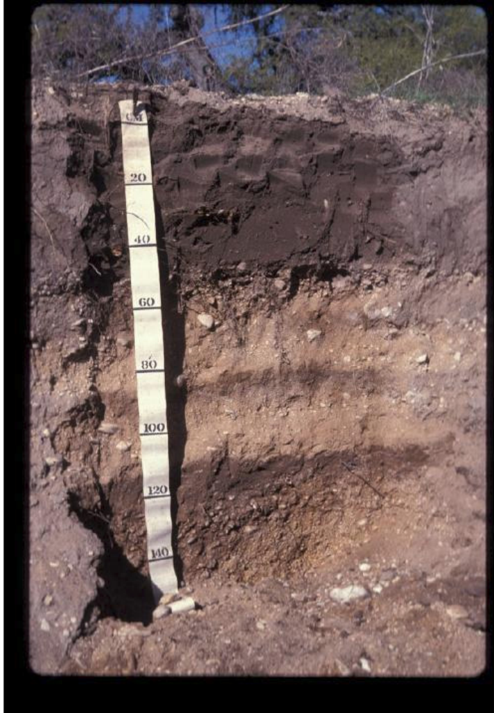
Figure 3.8 Illustration of soil horizons. In this frame, the soil horizons are very distinct and show the geological history of the soil.
