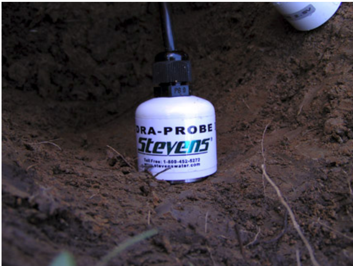
Figure 3.5 Hydra Probe Installed in undisturbed soil.
