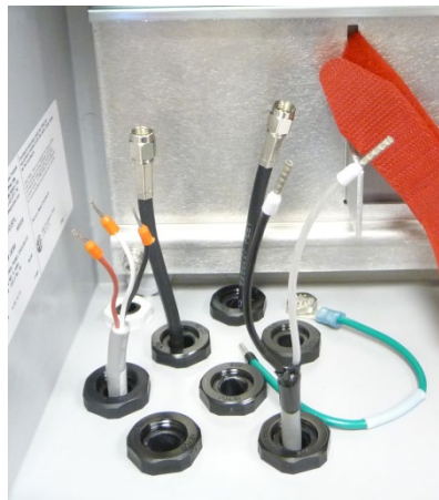
Figure 2-3: Gland replacement and inserted cables – externally mounted GPS
