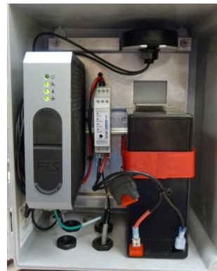
Figure 2-7: Solar Regulator status LEDs and final power connections (LT1-CELL shown)
