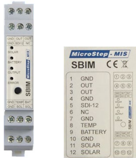
Figure 2-6: Solar regulator pin diagram
