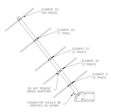
**Important:** Do not remove the brass adaptors that mount elements DE from the antenna.
