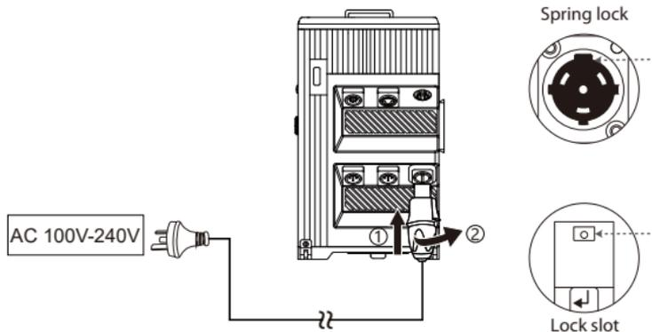
\* To disconnect the Neutrik® powerCon cable, pull back on the yellow release tab on the cable connector, and rotate the connector counter clockwise. Do not pull directly.
