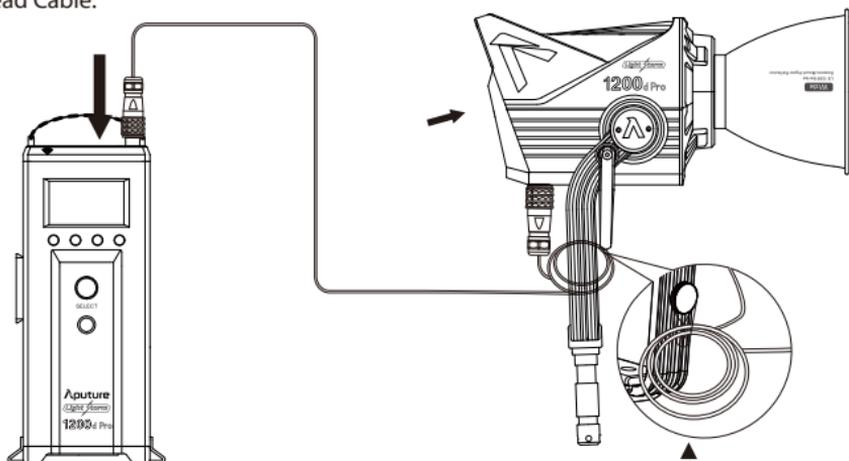
\* You can use the Cable relief hook to manage the connection line.
