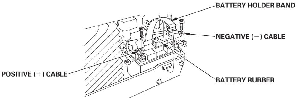
4. Remove the battery and the battery rubber from the battery tray.
