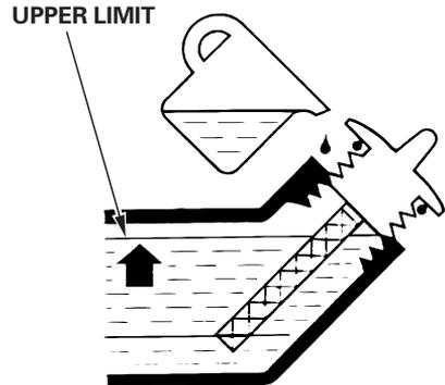
The Oil Alert system will automatically stop the engine before the oil level falls below safe limits. However, to avoid the inconvenience of an unexpected shutdown, check the oil level regularly.
