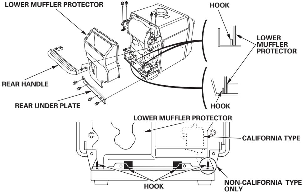
Install the lower muffler protector inside the hook securely.
