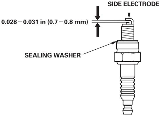
8. Check that the spark plug sealing washer is in good condition, and thread the spark plug in by hand to prevent cross-threading.
