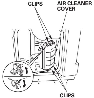
3. Check the foam air filter and paper air filter to be sure they are clean and in good condition. If the foam air filter is dirty, clean it as described on page 48. If the paper air filter is dirty, replace it with new one. Do not clean the paper air filter.
