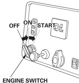
If the engine fails to start within 5 seconds, release the key, and wait at least 10 seconds before operating the starter again.
