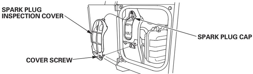
3. Remove the spark plug cap.
