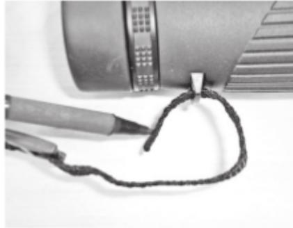
**STEP 2:** Thread the strap through the strap attachment lug on the binocular.
