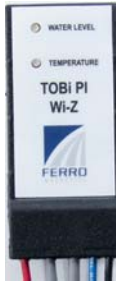
TOBi PI Wi-Z Wireless Communication between battery and charger and battery and computer.
