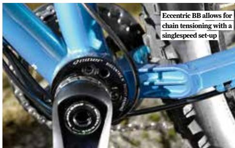
Eccentric BB allows for chain tensioning with a singlespeed set-up
