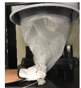
9- Pull the bag and place at the edge the band to create a new one. If necessary use two bands.
