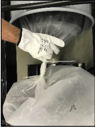
1 - Close the bag with two distanced bands.
