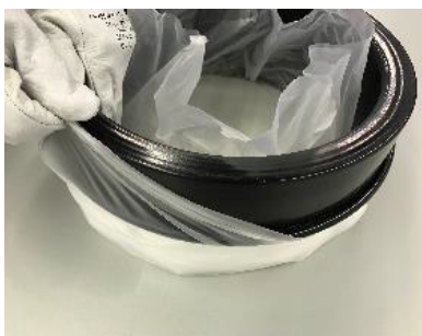
6- Pull the outer part of the bag to create the new one.
