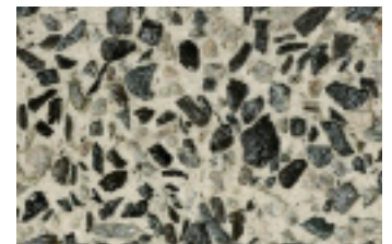
Large aggregate - remove more than 1/4"
