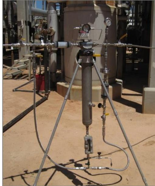
The GASCO test system allows for not only the quantification (and variability thereof) of all liquids entrained in a gas stream; it also allows for the isolation of *representative* contamination samples
