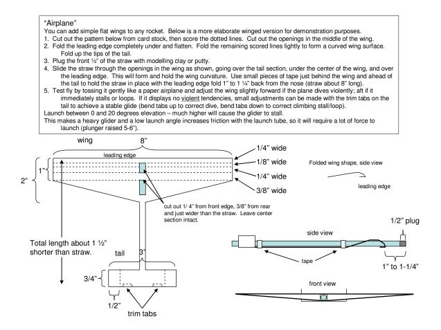
Below is a simpler glider pattern that can be cut from paper (enlarge so each glider pattern is 6" long, 5" wide). Folding the center section up and taping it forms a triangular fuselage beam that stiffens the paper enough to hold the wings straight. Use  $\frac{1}{2}$ " of clay in the nose and let the straw protrude 1-1/4" from the front wing edge for balance.
