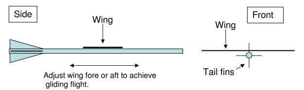
You can also make the above adjustment by taping a small ballast weight ( $\frac{1}{2}$ " of thick wire or a paperclip) to the bottom of the rocket tube. Move the weight aft if the rocket noses down. Move it forward if the rocket noses up too much.
