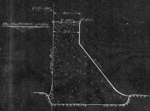
TYPICAL NON-OVERFLOW SECTION
