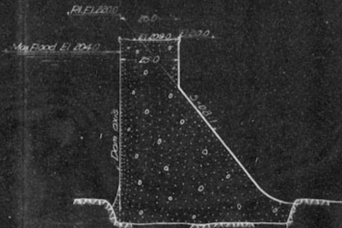
TYPICAL NON-OVERFLOW SECTION
