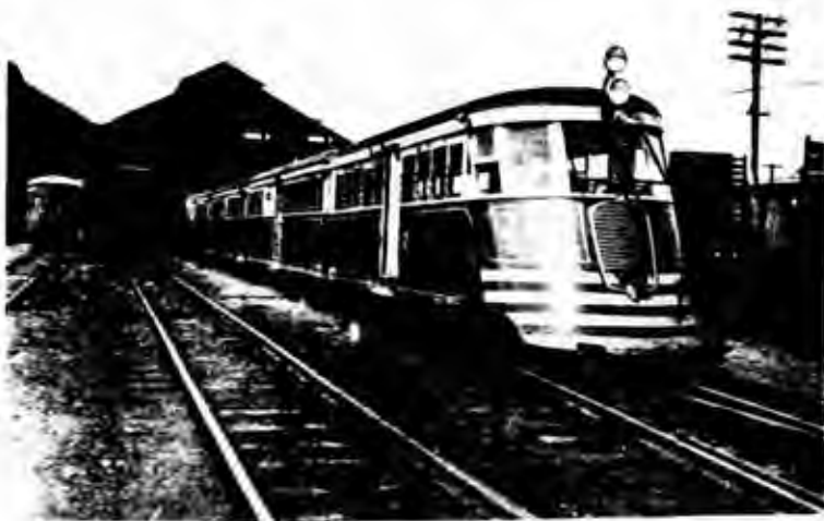
RAIL MOTOR TRAIN LEAVING MANILA TERMINAL STATION; RAIL MOTOR CAR POWERED WITH INTERNATIONAL 150 HORSE POWER MOTOR AND THREE TRAILERS. TOTAL SEATING CAPACITY OF TRAIN-150 PASSENGERS.
