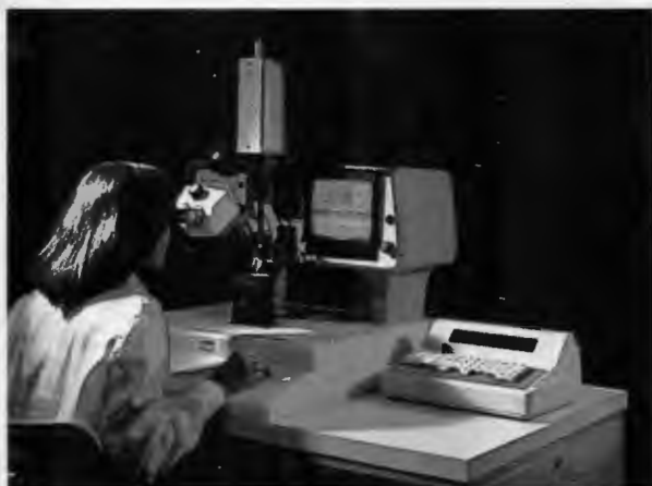
The HMC-2460 automatic wire bonder does much of the dirty work associated with hybrid circuit production—the tedious, rote tasks previously performed by human operators.
