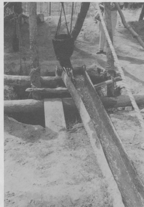
An ancient but ingenious device for raising water from a well is used in a Sahelian oasis to irrigate palms and vegetables.
