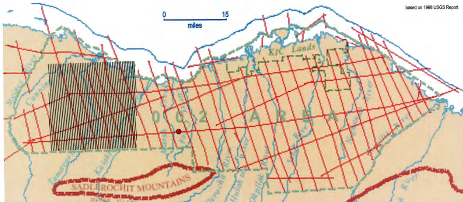
Figure 1. — Impact lines from 2-D seismic exploration in 1984-85. • Location of Figure 2 photographs. ||||| Typical line spacing for 3-D seismic exploration, overlaid on part of the coastal plain for comparison.
