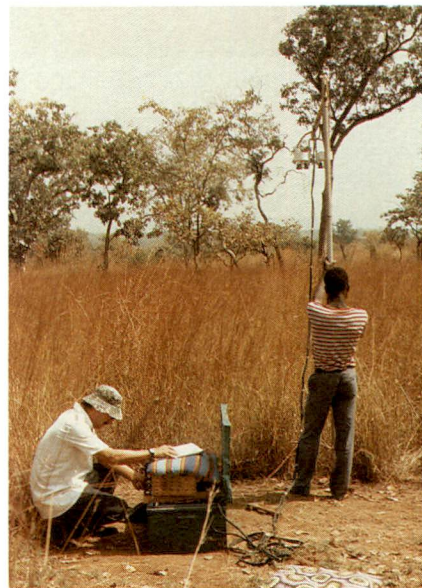
RIGHT: Scientists on an African field trip measure plant spectral reflectance for later comparison with satellite data.
