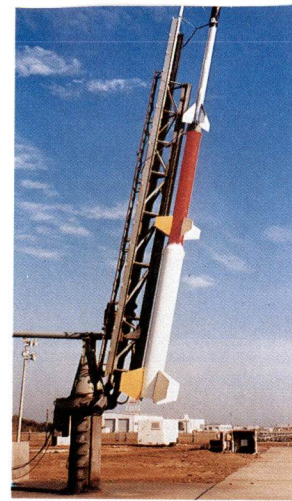
A sounding rocket is readied for launch at Wallops Flight Facility. These rockets fly near-vertical paths carrying scientific instruments to altitudes from 40 miles to hundreds of miles.
