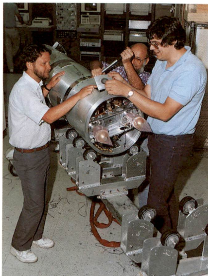
Final preparations for a spin balance test are conducted on a Black Brant IX sounding rocket payload section.
