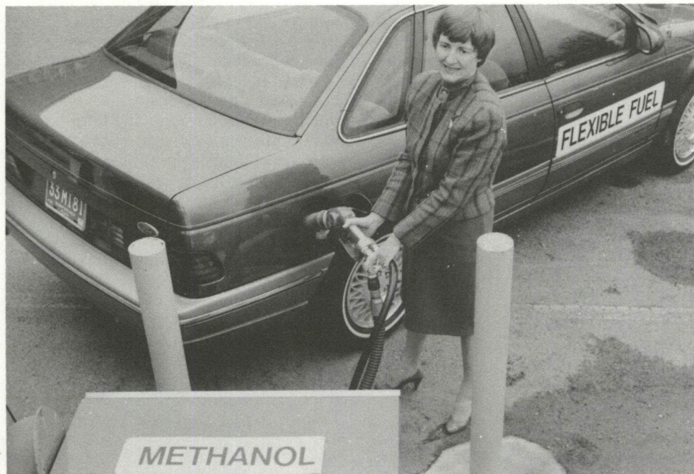
This Ford Taurus has been modified to run on methanol, ethanol, gasoline, or any combination of these fuels. Flexible-fuel cars may be a near-term means of alleviating the nation's air-quality problems. Shown is Roberta J. Nichols, who heads the company's Flexible Fuel Vehicle team.
