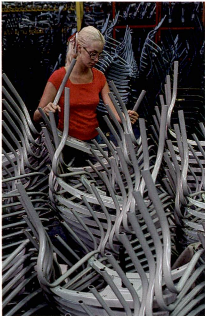
Chair frames are inspected at each stage of the manufacturing process.
