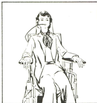
The MED Breath-Controlled wheelchair with Med-I-Cliner gives a quad total control of an electric wheelchair
