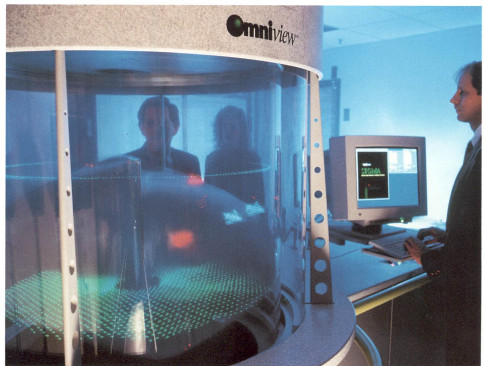
JNIDS' VISTA Volume Visualization System - developed with Texas Instruments. The 3-D laser disk display allows groups of analysts multiple views of moving scenarios, such as fighter tactics (above) or satellite orbital mechanics.
