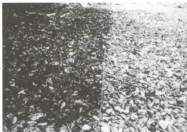
Test plots at Snug Harbor, Alaska, demonstrating the potential for use of bacteria capable of degrading oil in cleaning up of oil spills.
