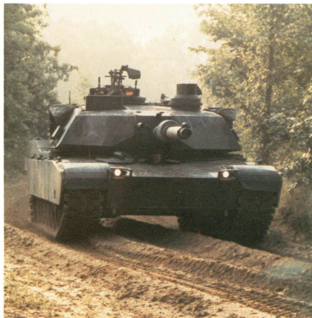
The Abrams M-1A1 main battle tank, work horse of the US armored force, has a 120-mm smooth bore gun, improved armor, and the commander's independent thermal viewer (CITV) in its latest variants.
