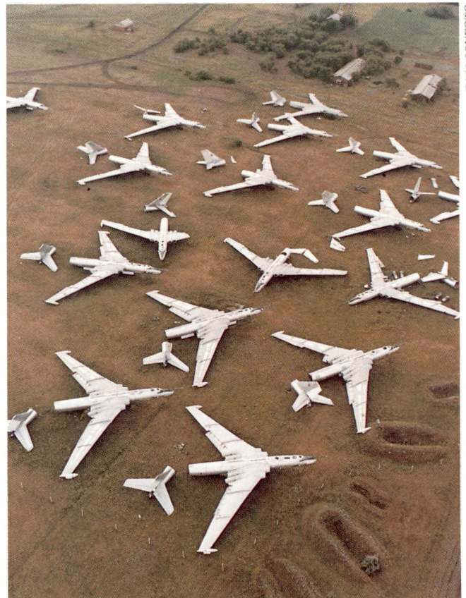
With their tail sections severed, obsolete M-4 Bison long-range bombers no longer count as part of the Soviet Union's manned strategic bomber force.
