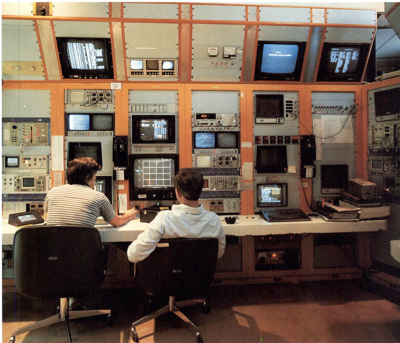
The main accelerator control room, where seven operators oversee the acceleration of a beam of protons and a beam of antiprotons to nearly the speed of light. When the beams are brought into collision, they create particles that cannot exist in more ordinary environments, providing new insights into the fundamental laws of nature.
