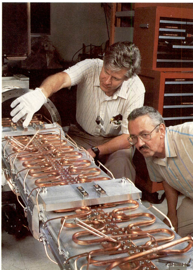
Part of the sophisticated stochastic cooling devices used in the complex process of producing and storing highly energetic, coherent bunches of antiprotons until enough accumulate to collide with protons about fifty thousand times a second in the Tevatron.
