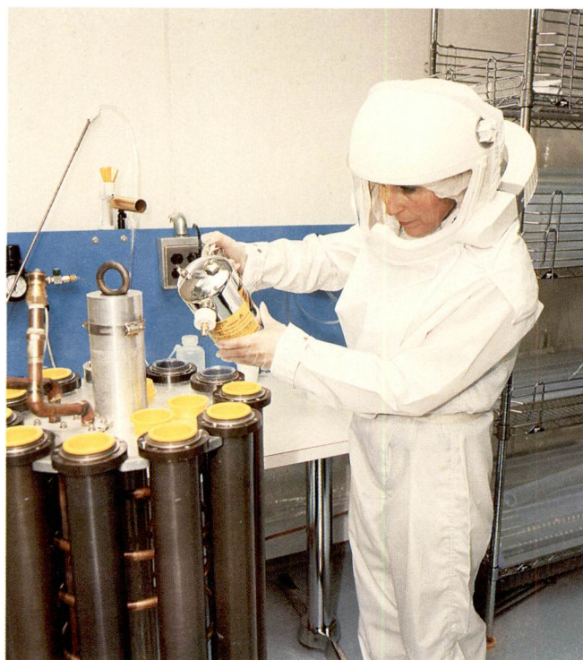
Some parts of an experiment are so sensitive that their fabrication and assembly require ultraclean conditions and operating-room precision. Here, scintillators are being made for the D-Zero detector. This colliding-beam experiment represents the combined effort of seventeen American universities, three American national laboratories, and laboratories in France and the Soviet Union.
