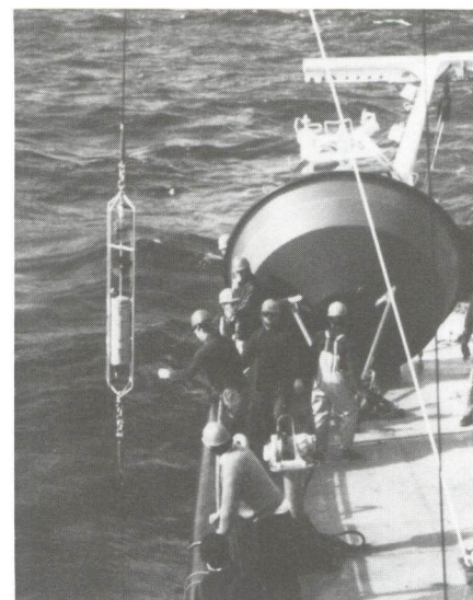
Biowatt researchers launch a multi-variable moored system instrument package and buoy.
