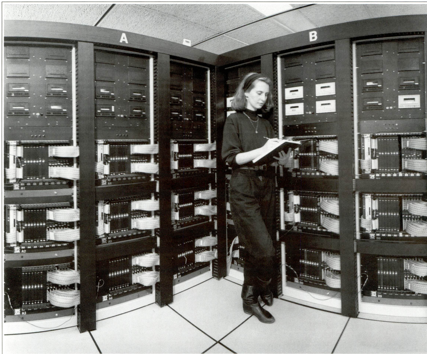
The ACPMAPS supercomputer was designed and constructed by Fermilab physicists and engineers. Fabricated from hundreds of independent, inter-
