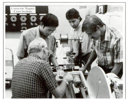
SSCL engineers and technicians wind the coil for a prototype corrector magnet.
