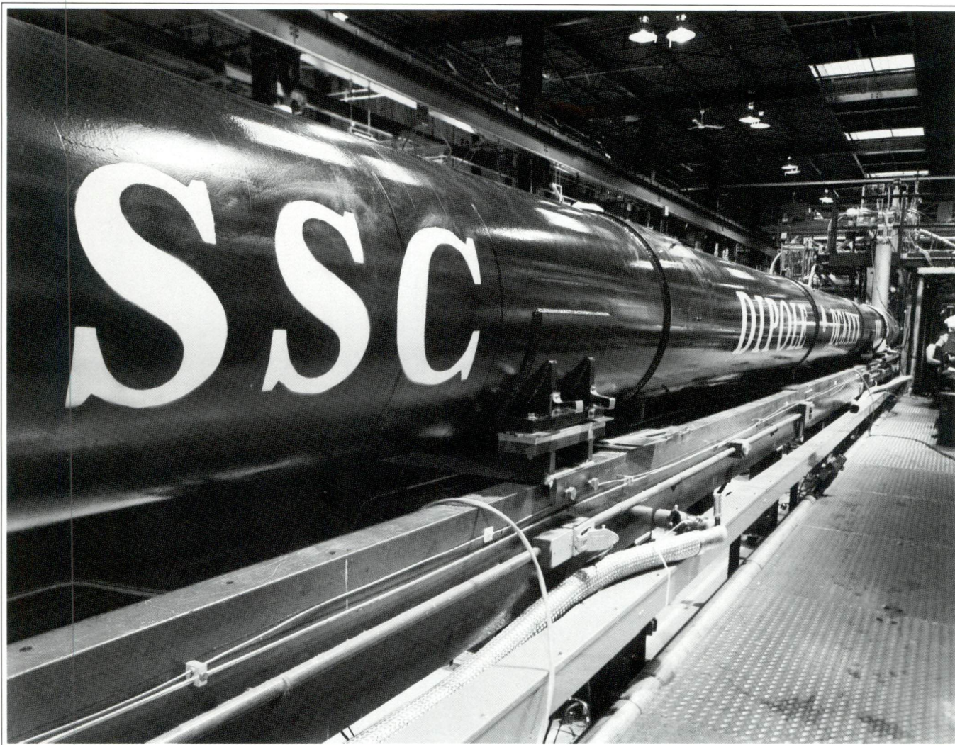
Prototype dipole magnets on a test stand at Fermilab. Successful tests of the redesigned 50-mm SSC
