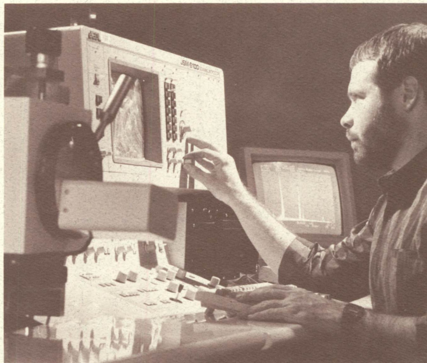
Electron Microscope. Powerful electron microscopes are used to analyze properties of the materials used in magnets for the SSC accelerator. The microscope magnifies up to 50,000 times and makes possible chemical and image analyses.
