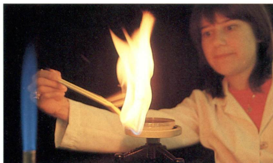
Researcher Barbara Karan-Tamir burns away the alcohol used to sterilize a wand prior to spreading bacterial colonies on an agar plate to evaluate genetically engineered organisms producing improved detergent enzymes.
