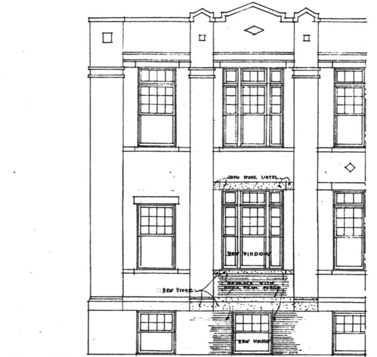
REVISED ELEVATION WITH ENTRANCE REMOVED AND WITH 2ND, 3RD AND BASEMENT WINDOWS SHOWN. PATCH ALL FINISHED WALL WHERE ORIGINAL WORK SHOWS DAMAGE. REPEAT THIS ELEVATION OPPOSITE END.
