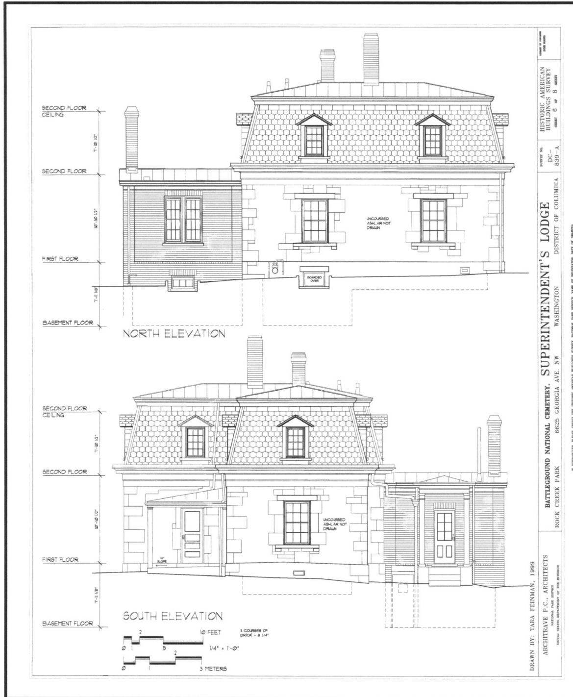
Superintendent's Lodge, North & South Elevations, Battleground National Cemetery, 1999 Source: Library of Congress, Historic American Buildings Survey, U.S. Historical, Cultural Collections
