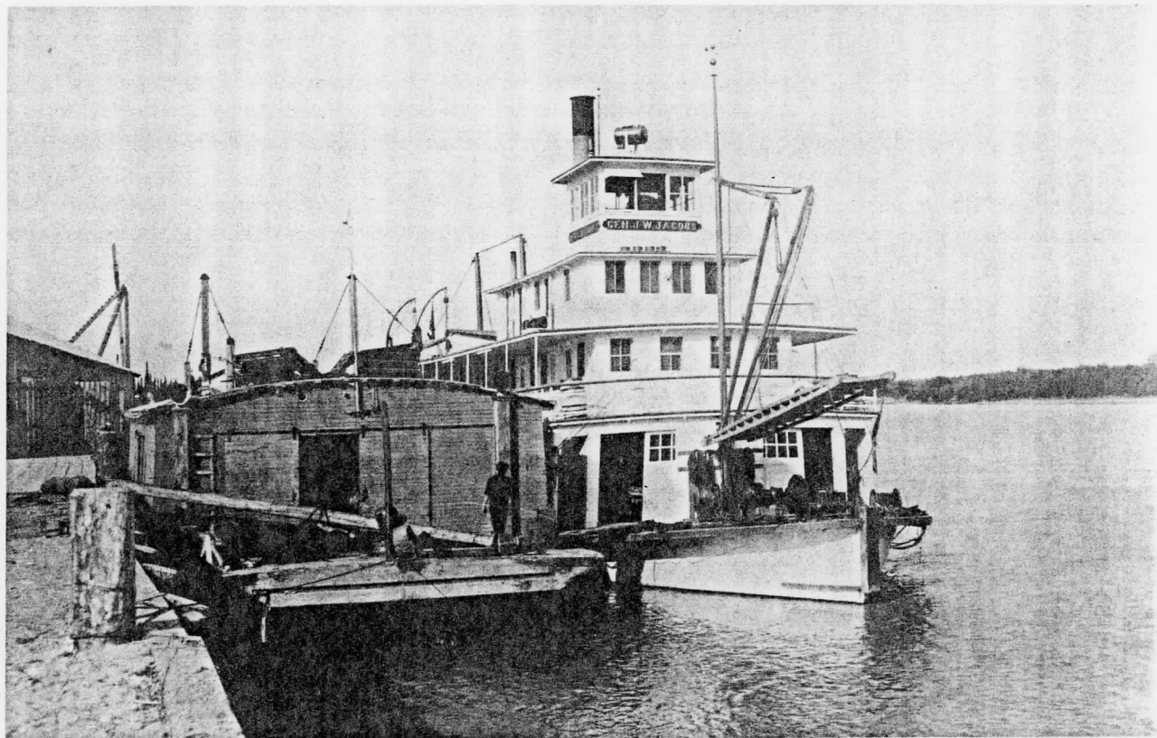
U.S. Army steamer General J. W. Jacobs loading cargo at Nenana, September 4, 1922. Note the old covered wooden barge, typical on the Yukon before 1940. (Anchorage Historical and Fine Arts Museum)
