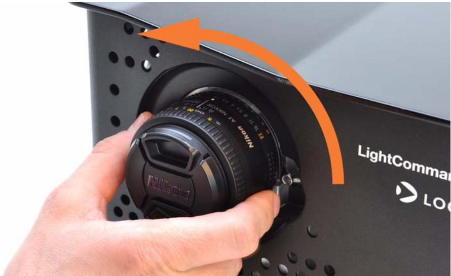
Figure 2.4 – Secure NIKKOR Lens to Lens Mount
