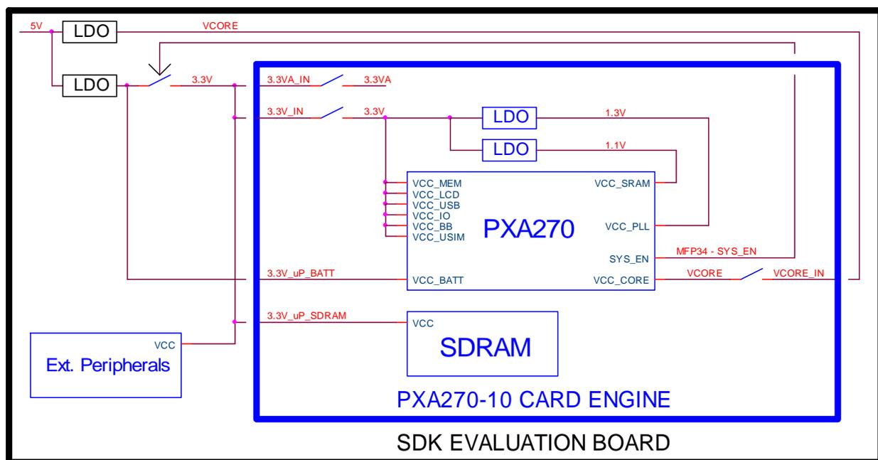
**Figure 3.1: SDK Power Supply Implementation**
