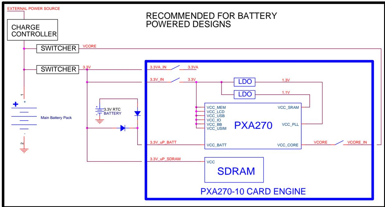
**Figure 3.2: Typical Block Diagram for Battery Powered Device**
