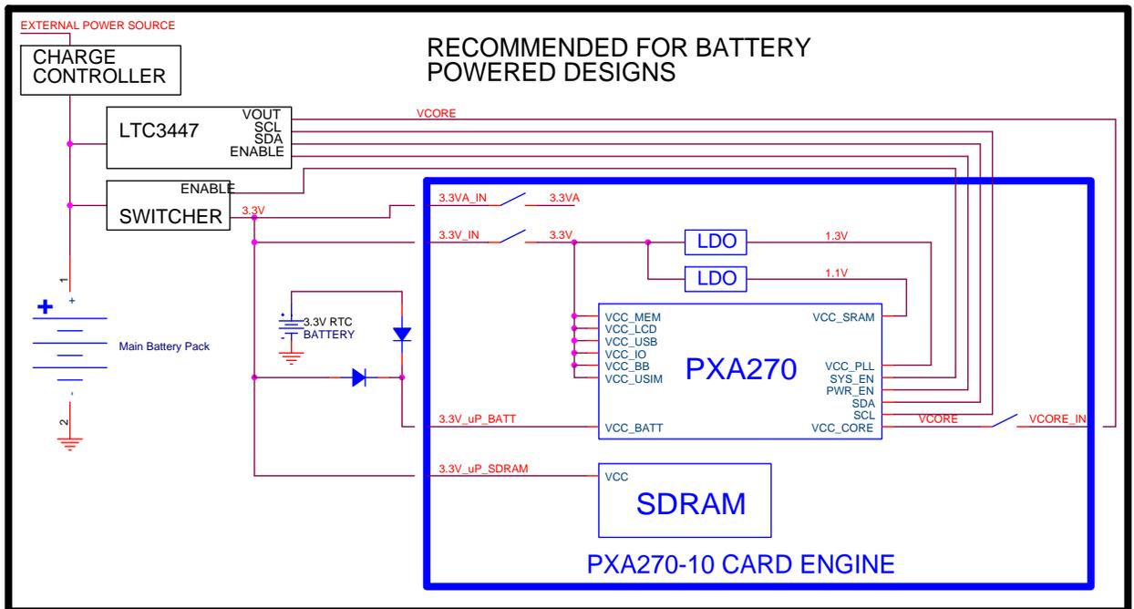
**Figure 3.4: Using IC Devices to Control Switching Regulation**
