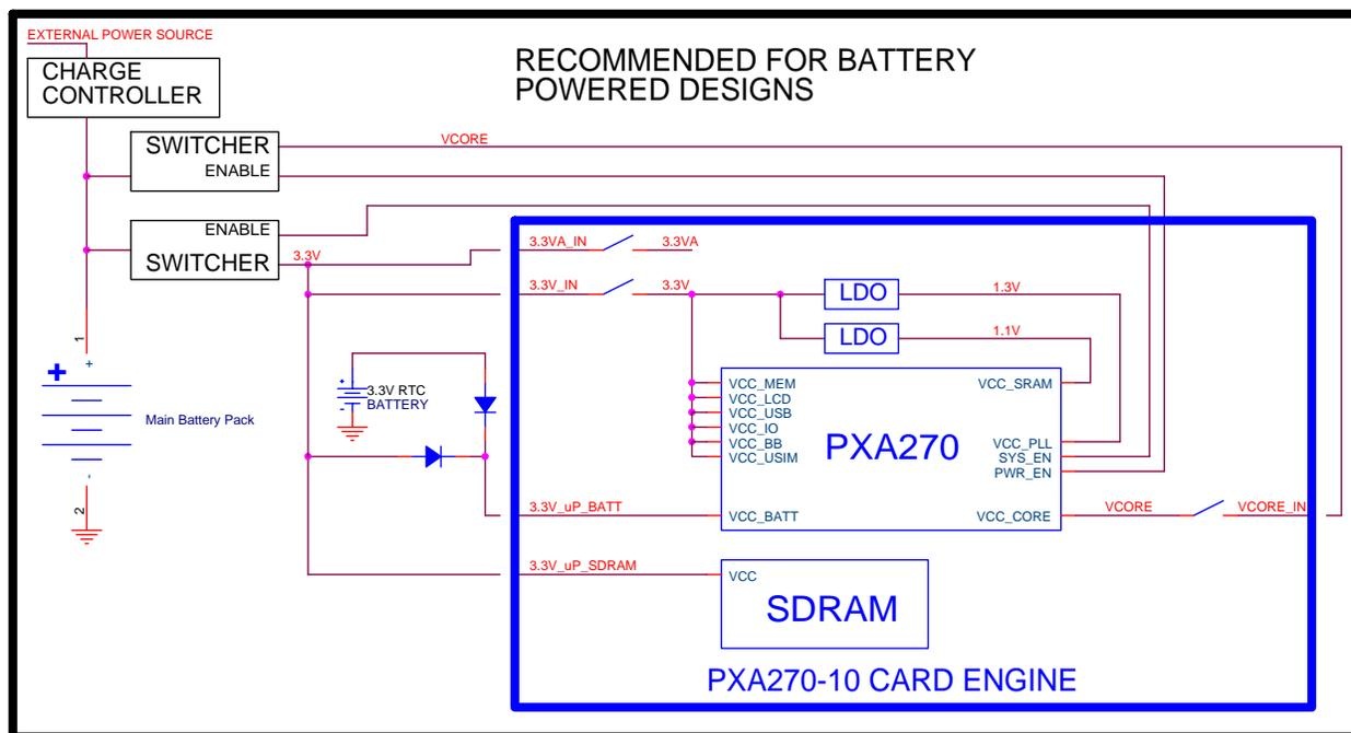
**Figure 3.3: Using PWR\_EN and SYS\_EN to Control Switching Regulator**
