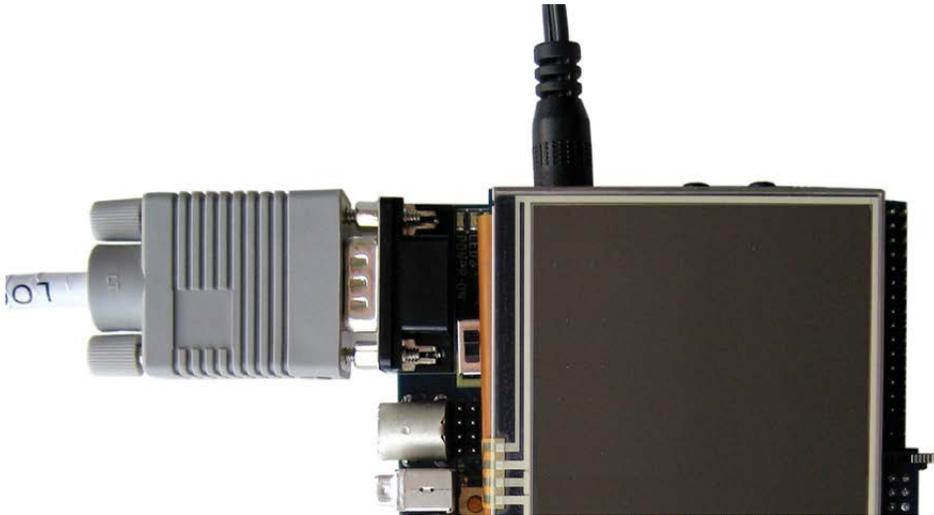
**Figure 3.1: Connect Serial Cable**
