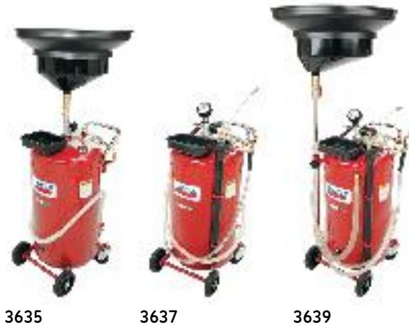
**Model 3635 gravity drain** has a portable upright configuration commonly used for collecting fluids under lift-mounted vehicles. It offers a 15 in. (381 mm) offset funnel that includes a removable filter screen and wide-mouth extension that increases the diameter to 24 in. (610 mm). Height is adjustable from 51 to 76 in. (1,3 to 1,9 m), not including the extension.
