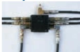
This photo depicts usage of adapters with checks, swivels, 90° fittings, swedge-on hose studs and reusable hose studs. Cumbersome.
