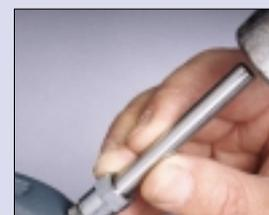
3. Seal and tighten Zerk-Lock™ using a hammer and staking tool
