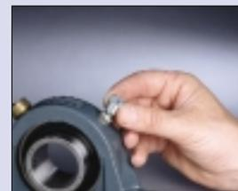
2. Place a Zerk-Lock™ onto the fitting
