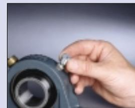
2. Place a Zerk-Lock™ onto the fitting
