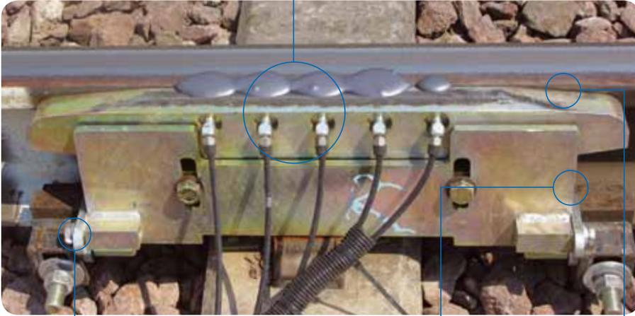
*Mounting brackets allows bar to be folded out of the way for routine track maintenance.*
