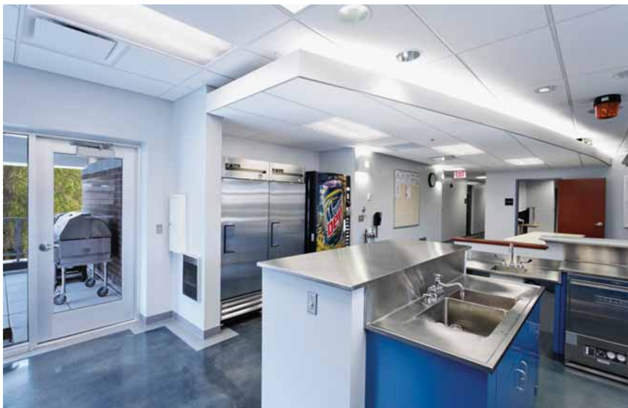
Cincinnati Fire Station No. 9 incorporates an ADA compliant sink mounted at 34 inches and with a depth of 6.5 inches, as well as a standard sink.
