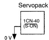
When S-ON is not used, this short-circuit wiring can be omitted.
