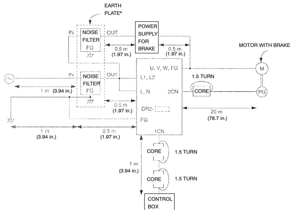
\* When earth plate is not used, polish the mounted noise filter part with sand paper to expose the metal. Then, ground the noise filter securely on the panel.
