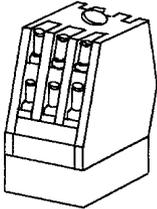
Turns the main power ON or OFF. Use a surge suppressor for the magnetic contactor.
