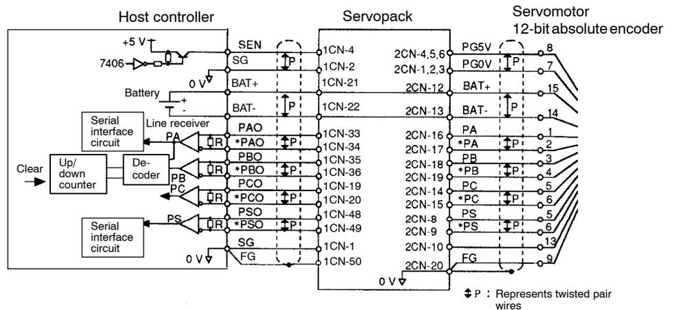
Line Receiver Used: SN75175 or MC3486 manufactured by Texas Instruments Inc.
