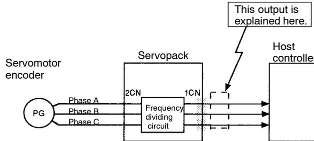
The output circuit is for line driver output. Connect each signal line according to the following circuit diagram.
