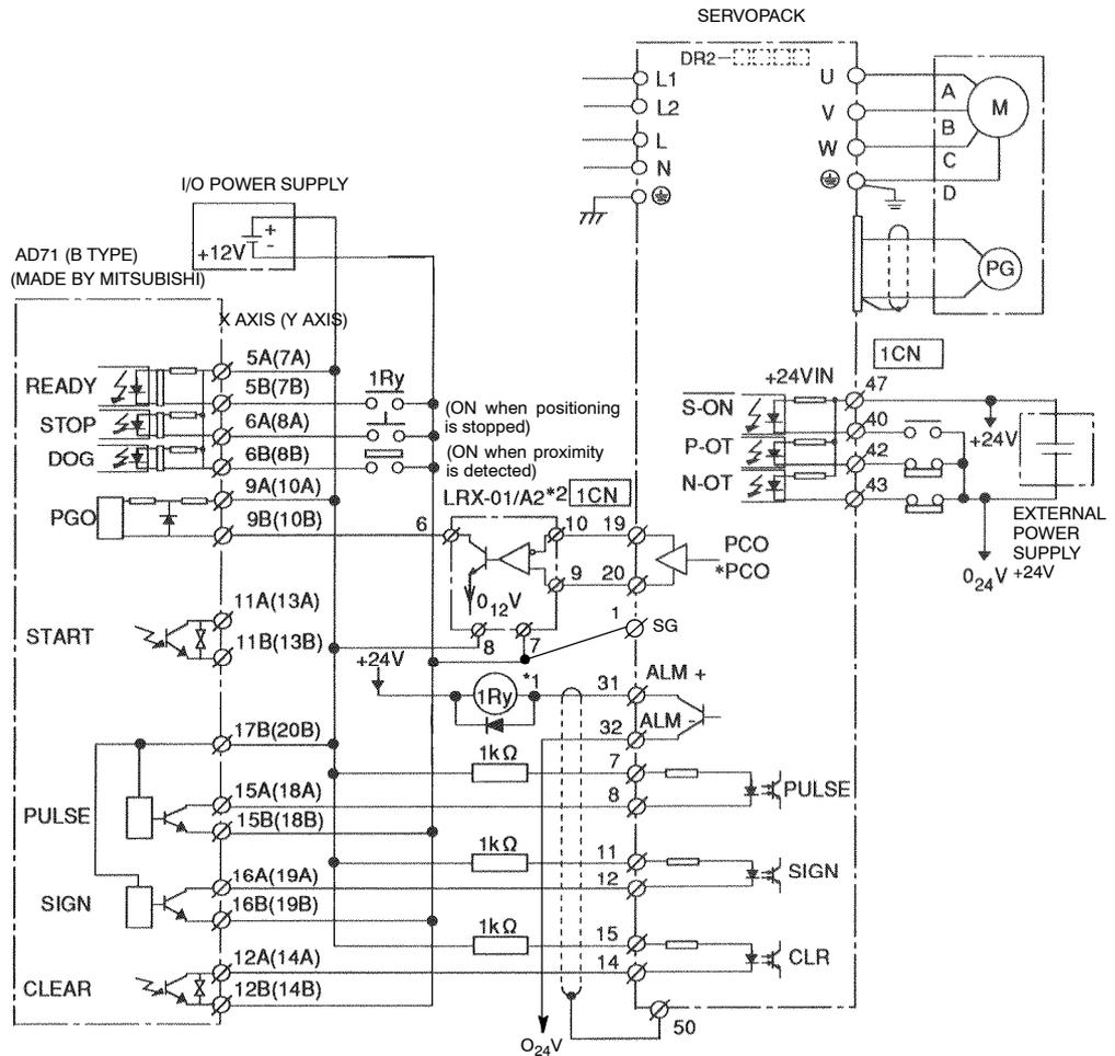
\*1 These signals are output for approximately two seconds when the power is turned ON. Take this into consideration when designing a power ON sequence. Relay 1Ry is used to stop main circuit power supply to Servopack.
