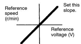
The factory setting is 500 [rated speed (3000 r/min)/6 V = 500].
