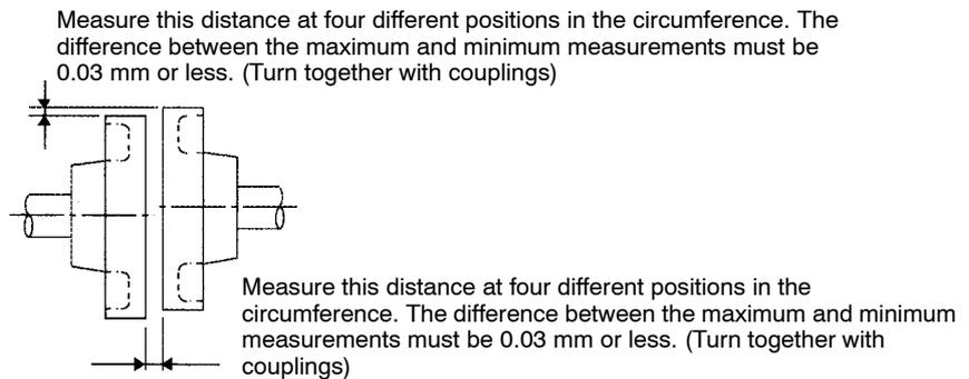
**NOTE** If the shafts are not aligned properly, vibration will occur, resulting in damage to the bearings.
