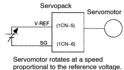
**When a host controller such as a programmable controller performs position control, it may be difficult to directly input the speed reference voltage. In this case, constant voltage reference should be input once to ensure correct operation.**
