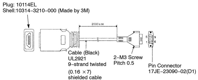
Note: Fold back the cable shielding at each end of the cable and secure it with clamp.
