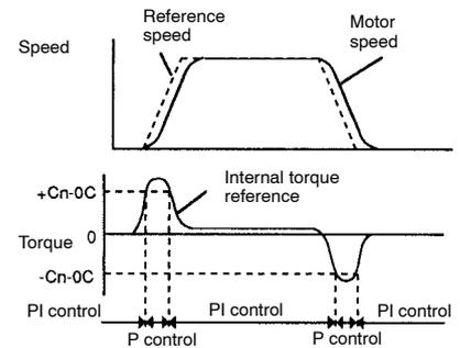
If a mode switch is not used and PI control is always performed, torque may enter a saturation state during acceleration or deceleration, causing the motor speed to have overshoot or undershoot.
