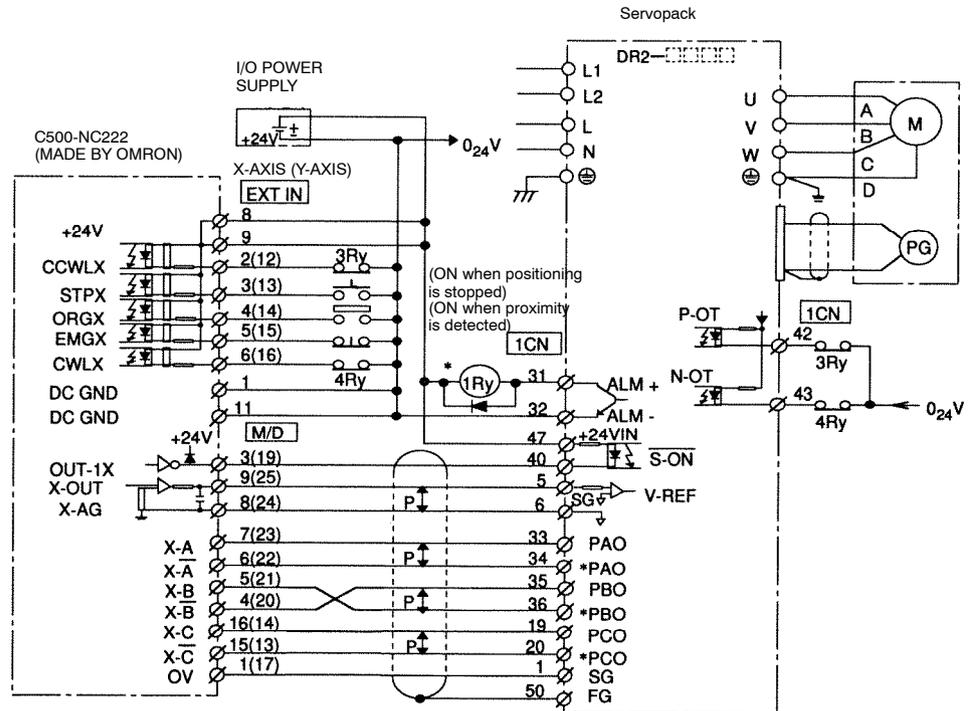
\* These signals are output for approximately two seconds when the power is turned ON. Take this into consideration when designing a power ON sequence. Relay 1Ry is used to stop main circuit power supply to Servopack.
