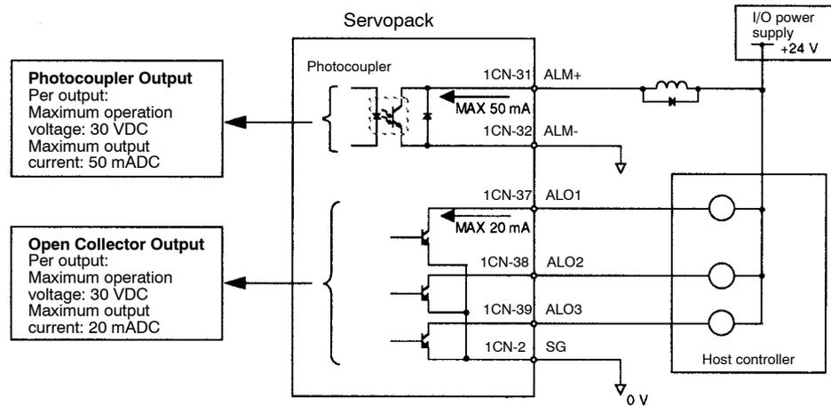
Provide an external I/O power supply separately. There are no DC power available from Servopack for output signals.
