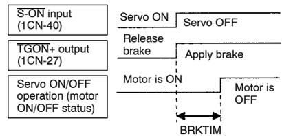
With the standard setting, the servo is turned OFF when  $\overline{\text{TGON+}}$  signal (brake operation) is output. The machine may move slightly due to gravitation. This movement depends on machine configuration and brake characteristics. If this happens, use this user constant to delay servo OFF timing to prevent the machine from moving.
