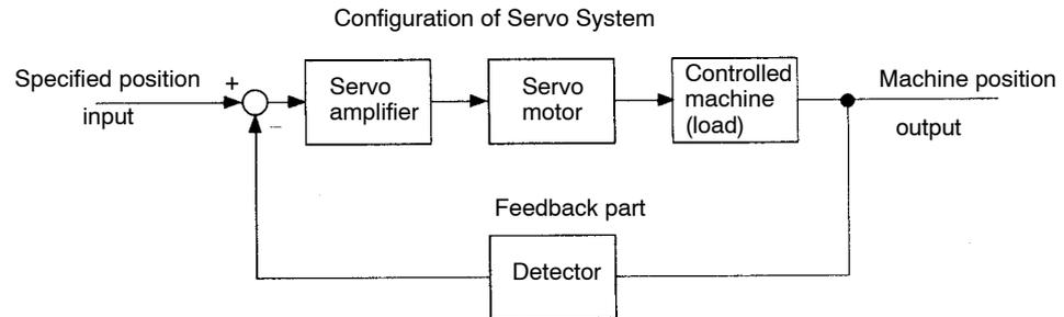
This servo system is an automatic control system that detects the machine position (output data), feeds back the data to the input side, compares it with the specified position (input data), and moves the machine by the difference between the compared data.
