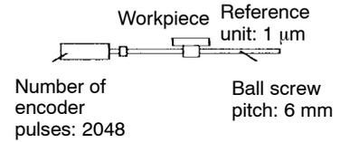
Machine conditions and reference unit must be defined for the electronic gear function beforehand.
