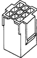
Encoder Connector for Servopack End of Cable
