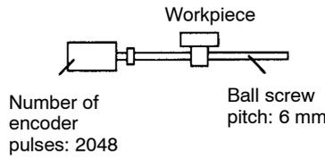
To move a workpiece 10 mm,
