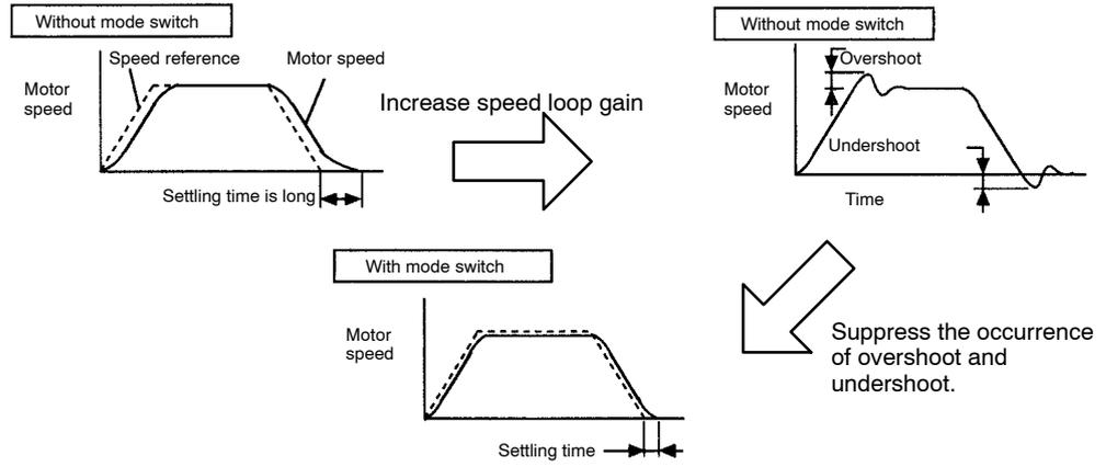
**When Acceleration Is Used as a Detection Point of Mode Switch**
