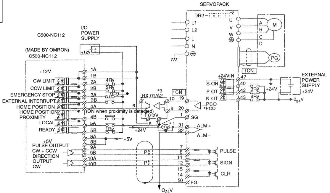
\*1 These signals are output for approximately two seconds when the power is turned ON. Take this into consideration when designing a power ON sequence. Relay 1Ry is used to stop main circuit power supply to Servopack.
