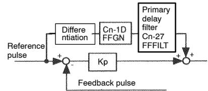
This user constant is set to apply feed-forward frequency compensation to position control inside the Servopack.
