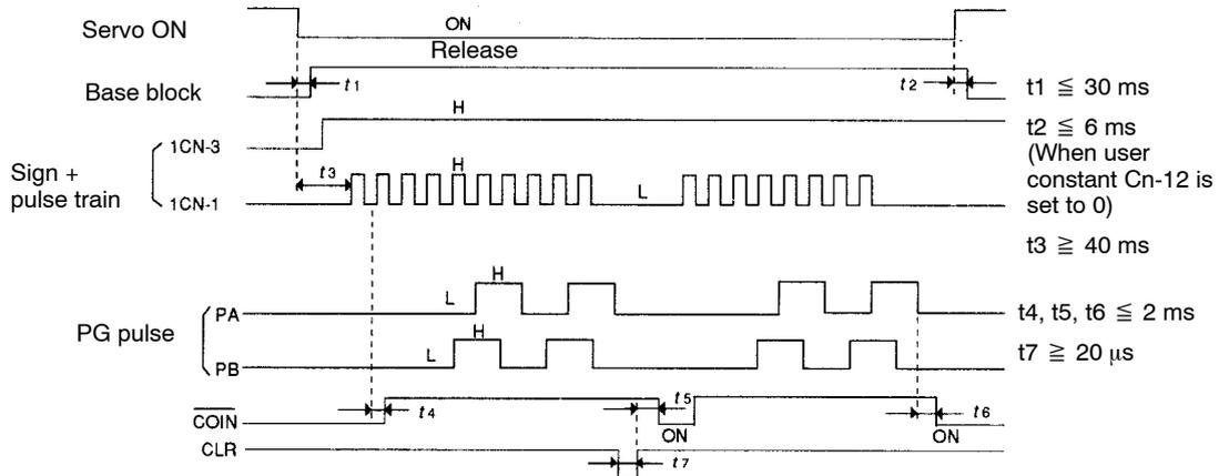
**Note** The interval from the time the servo ON signal is turned ON until a reference pulse is input must be at least 40 ms. Otherwise, the reference pulse may not be input. The error counter clear (CLR) signal must be ON for at least 20  $\mu\text{s}$ . Otherwise, it becomes invalid.
