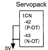
Specifies "1" when external short-circuit wiring is to be omitted.
