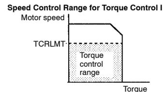
For torque control I, set bits A and B of memory switch Cn-01.
