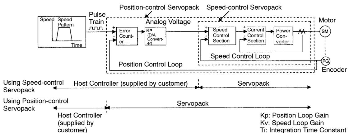
**Note:** A position-control Servopack has no D/A converter for speed reference output. This conversion is handled by internal calculations.
