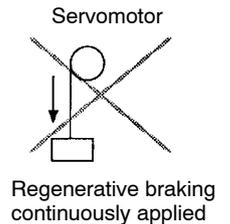
**The Servomotor cannot be operated by turning the power ON and OFF.**
