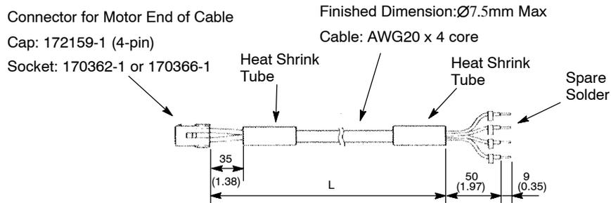
b) Cables For Motor With Brake (with connector and AMP terminals)
