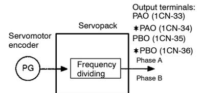
The number of output pulses per revolution is set in this user constant. Set this value according to the reference unit of the machine or controller to be used.
