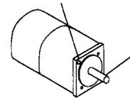
Do not connect anything to the motor shaft (no-load status).
