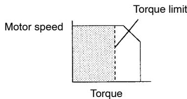
Note that too small a torque limit value will result in torque shortage at acceleration or deceleration.
