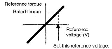
The factory setting is 30, so the rated torque is 3 V (30 x 0.1).
