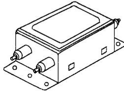
Install to eliminate external noise from the power lines.
