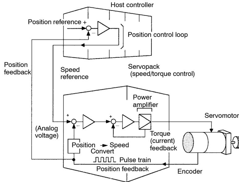
As shown in the figure above, a position control loop is formed in the host controller. The host controller compares a position reference with a position feedback signal and sends processing results to the Servopack as a speed reference.
