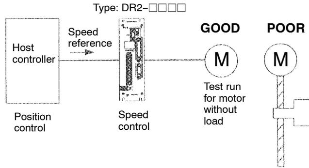
**NOTE** Check the motor operation with the motor disconnected from the machine. If the host controller does not perform position control correctly, the motor may run out of control.
