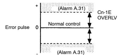
If the machine permits only a small position loop gain value to be set in Cn-1A, an overflow alarm may arise during high-speed operation. In this case, increase the value set in this user constant to suppress alarm detection.
