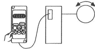
Set the motor speed (JOG speed) in this user constant when motor is operated using the digital operator.
