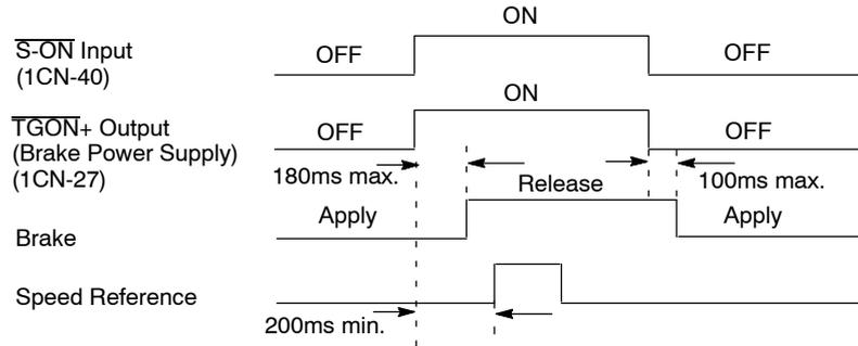
Min. 200ms is required between brake power ON ( $\overline{\text{TGON+}}$ ) and speed reference input. As for the brake holding timing at servo OFF, refer to 4) and 5) shown below.
