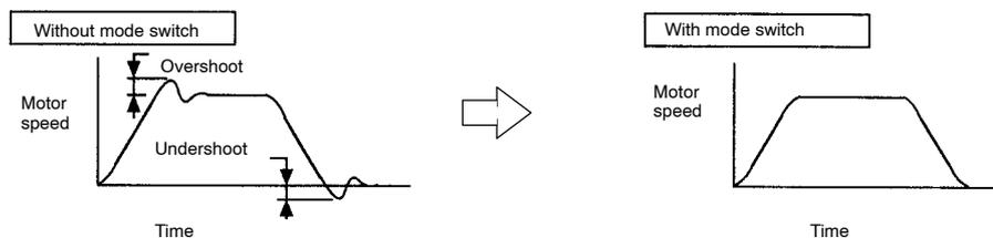
**When Speed Reference Is Used as a Detection Point of Mode Switch**
