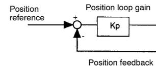
Increasing the position loop gain value provides position control with higher response and less error. However, there is a certain limit depending on machine characteristics.
