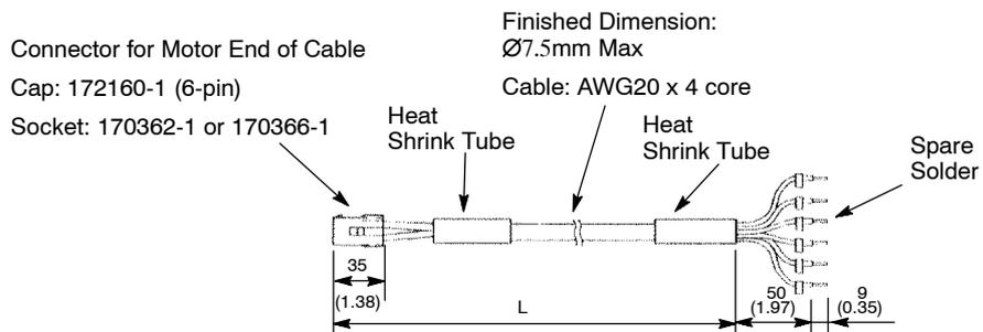
c) Cables For Motor Without Brake
