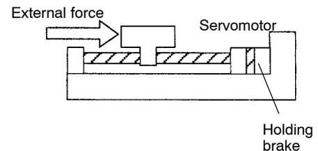
**NOTE** To prevent faulty operation caused by gravity (or external force), first check that the motor and holding brake operate normally with the motor disconnected from the machine. Then, connect the motor to the machine and conduct a test run.
