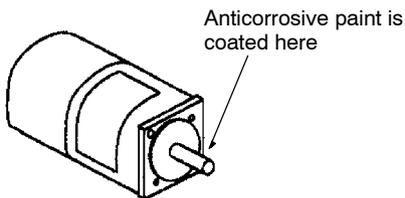
**NOTE** Avoid getting thinner on other parts of the Servomotor when cleaning the shaft.
