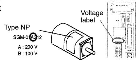
**Always use the SGM/SGMP Servomotor and DR2 Servopack in pairs.**
