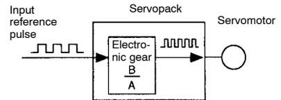
$$\text{Electronic gear ratio } \left(\frac{B}{A}\right) = \frac{\text{Cn-24}}{\text{Cn-25}}$$
