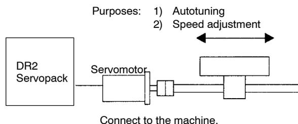
**NOTE** Before proceeding to step 2, repeat step 1 (conducting a test run for the motor without load) until you are fully satisfied that the test has been completed successfully. Operation faults that arise after the motor is connected to the machine not only damage the machine but may also cause an accident resulting in injury or death. Therefore, all items including user constants setting and wiring should be tested as conclusively as possible before step 1 is complete.
