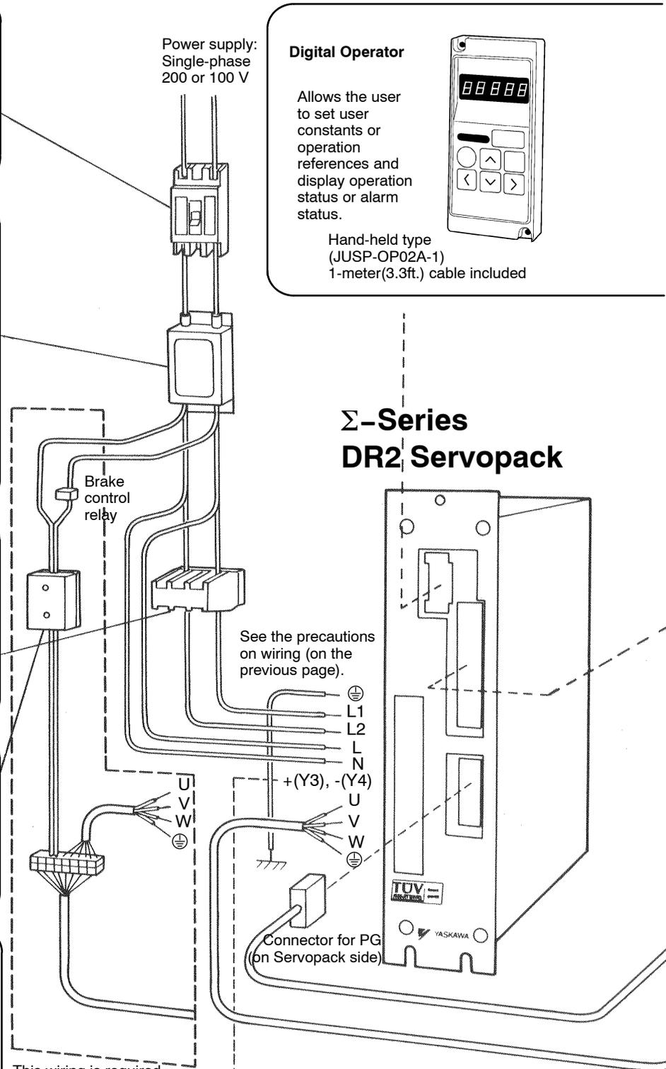
This wiring is required only for a Servomotor with brake
