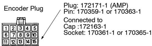
Motor Wiring Specifications
