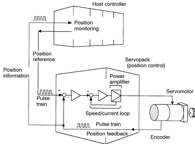
The host controller can send a position reference (pulse train) to the Servopack to perform positioning or interpolation. This type of Servopack contains a position control loop.
