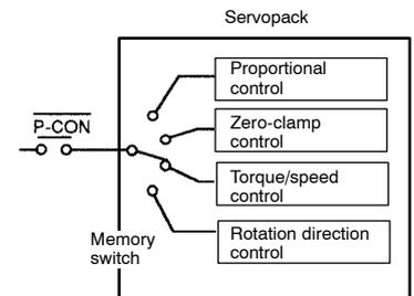
The function of  $\overline{\text{P-CON}}$  signal varies according to the memory switch setting.
