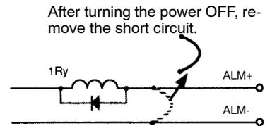
After turning the power OFF, remove the short circuit.
