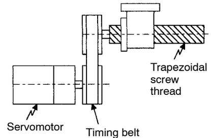
To develop an excellent servo system, it is important to select a rigid drive system that has no play.
