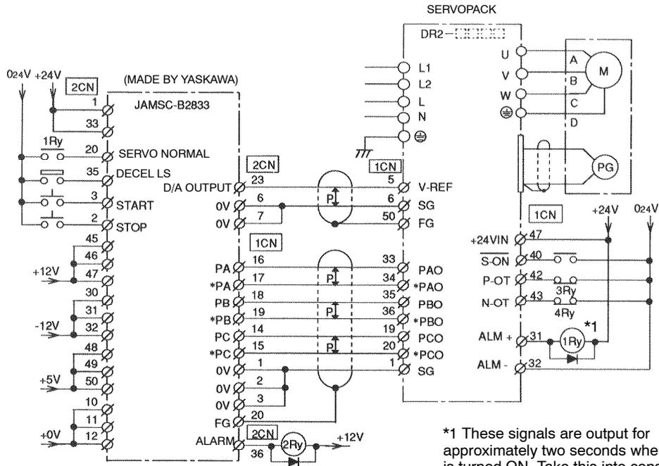
\*1 These signals are output for approximately two seconds when the power is turned ON. Take this into consideration when designing a power ON sequence. Relay 1Ry is used to stop main circuit power supply to the Servopack.
