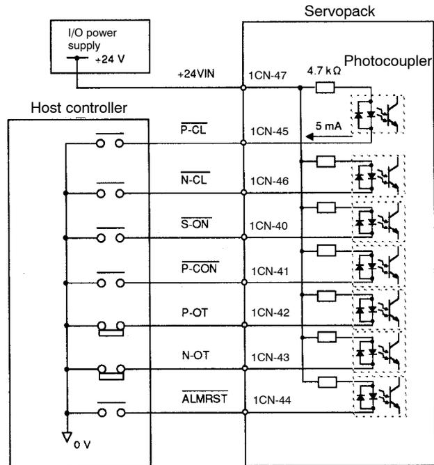
**Note** Provide an external I/O power supply separately. There are no power terminals to which the DR2 Servopack outputs signals externally.
