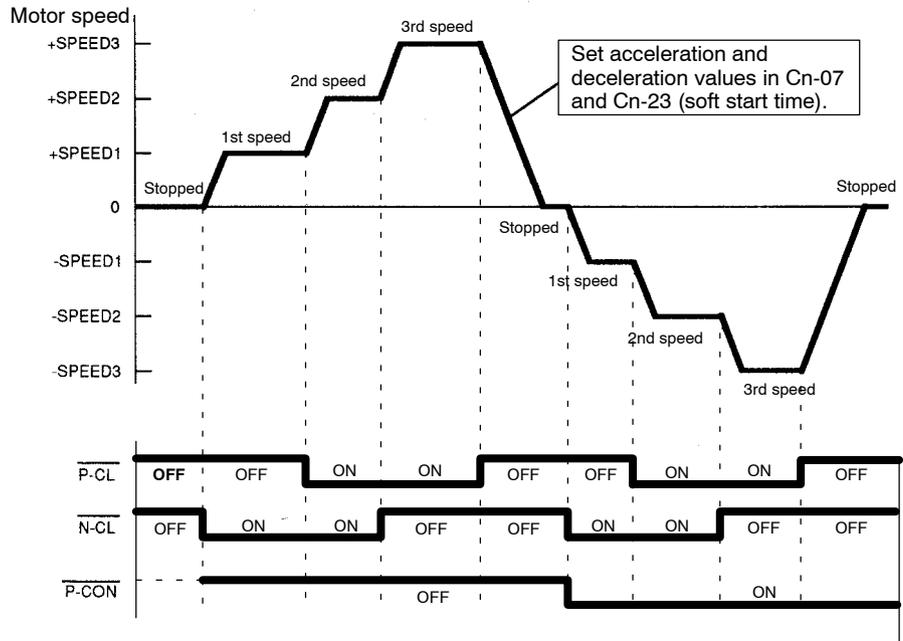
**Note** For the position control, the soft start function is available only when contact input speed control is used. The soft start function is not available when pulse reference input is used.
