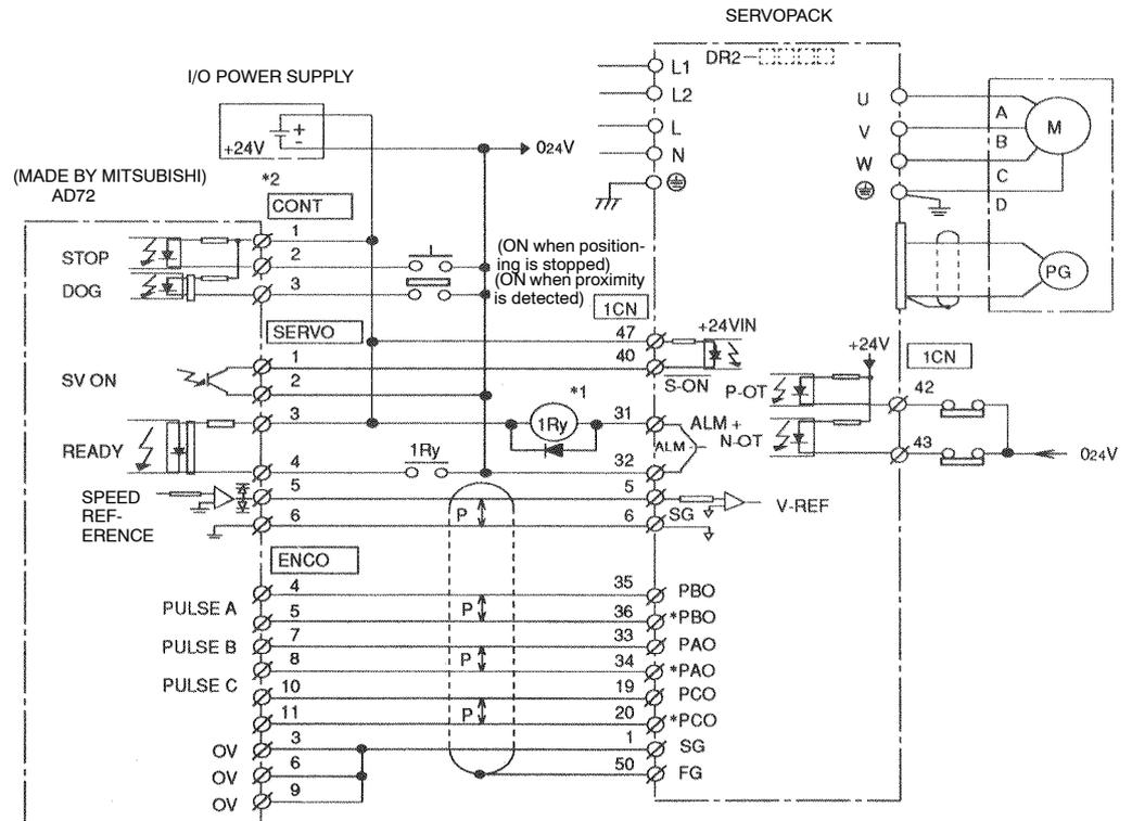
\*1 These signals are output for approximately two seconds when the power is turned ON. Take this into consideration when designing a power ON sequence. Relay 1Ry is used to stop main circuit power supply to Servopack.
