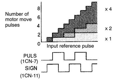
**Example of I/O Signal Generation Timing**
