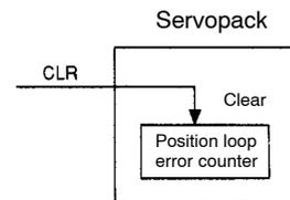
Bit A of memory switch Cn-02 can be set so that the error counter is cleared only once when the leading edge of an input pulse rises.
