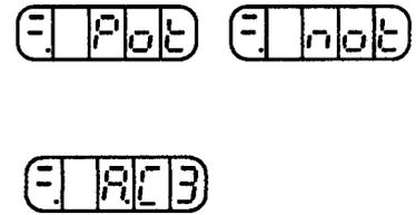
If an alarm display appears on the LED as shown in the figure above, the power supply circuit, motor wiring or encoder wiring is incorrect. In this case, turn the power OFF, then correct the problem.
