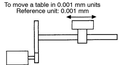
Determine the reference unit according to machine specifications and positioning accuracy.
