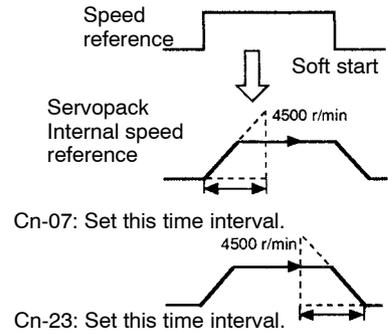
3) Contact input speed control performs the following operation.
