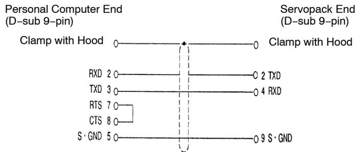
5) Cable for connecting Servopack and NEC PC-98 half-pitch connector
