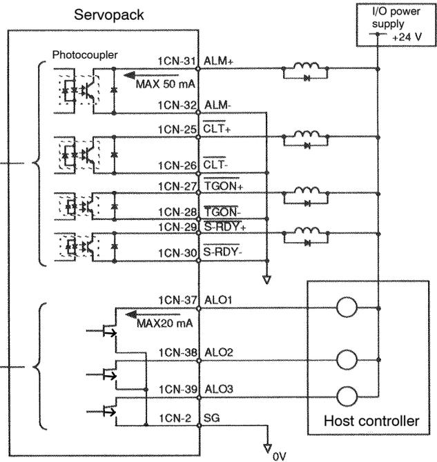
**Note** Provide an external I/O power supply separately. There are no power terminals to which the DR2 Servopack outputs signals externally. Yaskawa recommends that this external power supply be the same type as for the input circuit.
