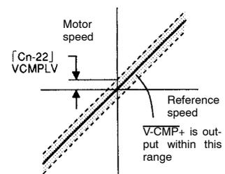
Example: When preset value is 100 and reference speed is 2000 r/min.
