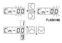
3. Press the ENTER key to display the data for the memory switch parameter selected in step 2.
