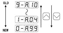
\* The alarm trace back data is not eliminated by the alarm reset or even by the turning off of the servopack power. (No interference with operation.)
