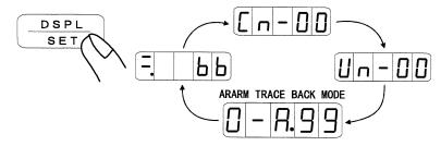
2. Using the and keys will display higher or lower alarm numbers, with the information about the alarms also displayed. The higher the number on the left, the older the alarm.
