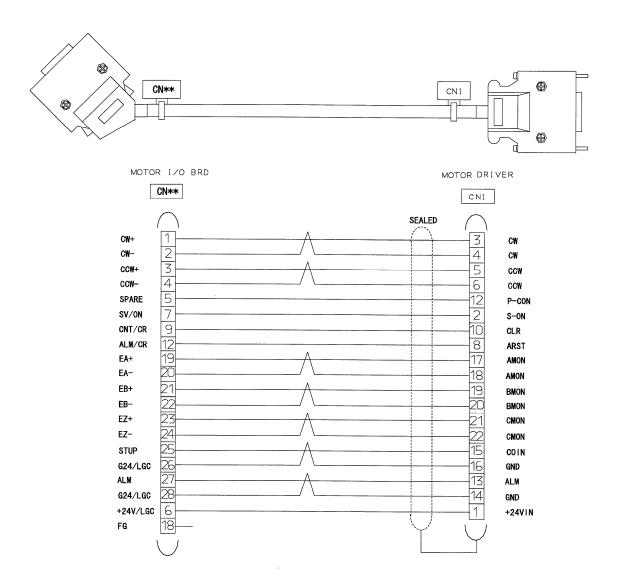
The CN\*\* designation of the motor I/O board shows that spinner 1 is connected to CN17, spinner 2 to CN18, spinner 3 to CN19, and spinner 4 to CN20.
