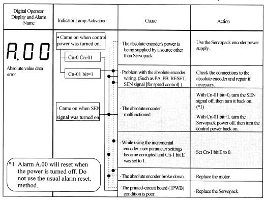
: Since incremental encoders are used, the alarm does not apply to the shaded part.
