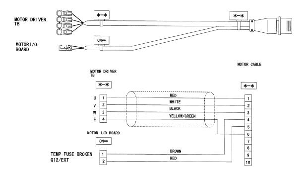
The \*-\* designation of the motor driver TB shows the block number and module number. These are connected to the 1, 2, 3, and 4 motor driver terminal blocks.
