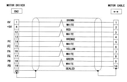
The \*-\* designation of the motor cable shows the block number and module number. These are connected to the 1, 2, 3, and 4 spin motor encoder cable.
