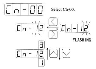
3. Press the ENTER key to display the current data for the Cn-00 user parameter.
